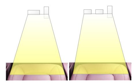
**Note:** The width at the pedals could move one way or the other but this width must be maintained and a straight line from the side of the seat to each side of the foot well needs to be maintained.
